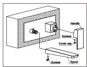
7.Install the spout to the valve with screws and check if there is any leakage. And then install the handle to the valve with screws and put back the cover cap. Installation
